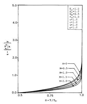
Fig. 1 Fluid-phase temperature profiles.
