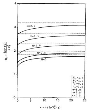
Fig. 2 Wall heat transfer vs  $\varepsilon$ .
